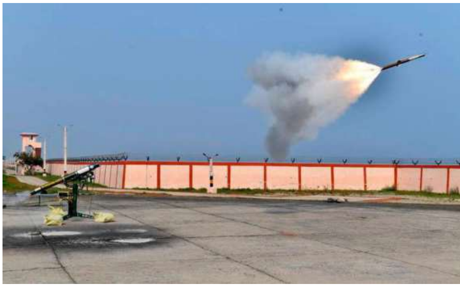
POINT TO POINT. The Defence Research and Development Organisation conducted two successful flight tests of Very Short-Range Air Defence System (VSHORADS) missiles from a portable launcher. These tests were carried out from Integrated Test Range, Chandipur, off the coast of Odisha, over two days from Wednesday. VSHORADS, a man-portable air defence system, managed to hit high speed unmanned aerial targets under different interception scenarios XIG/DEFPRODINDIA
